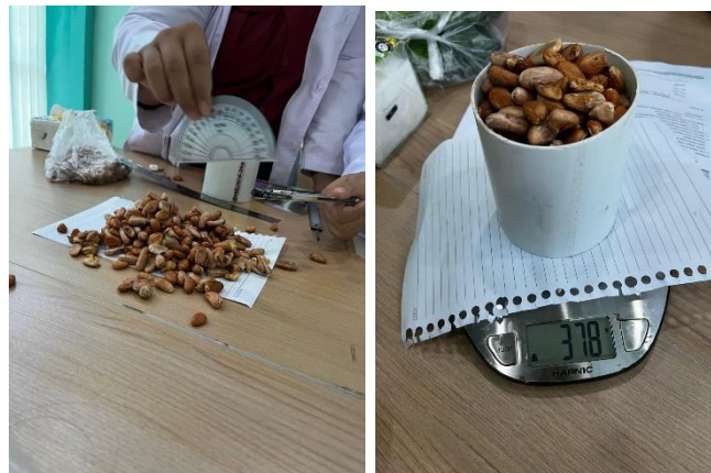
Figure 1. (a) measuring the slope (b) weighing the mass of ripe cocoa beans
