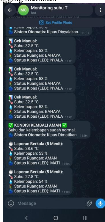
Picture3. Evaluation Results of Notification Delivery and Automatic Control on the Telegram Application
