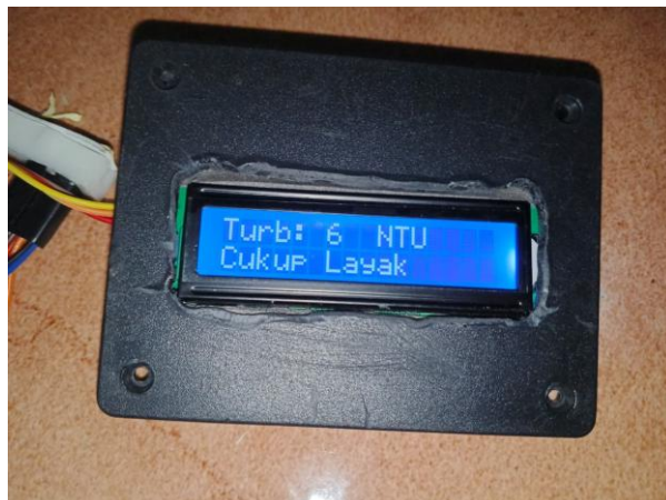
Figure 8. Test results if the water is not too acidic and its validity
