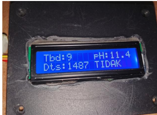
Figure 10. Test results of 3 sensors showing unsuitable water conditions
