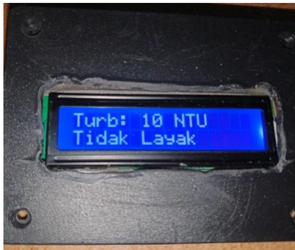
Figure 5. Test results if the water is too cloudy
