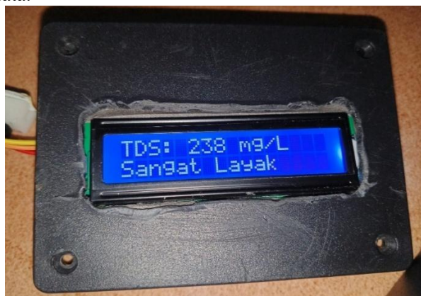
Figure 1. Results of testing dissolved substances in the very suitable category
