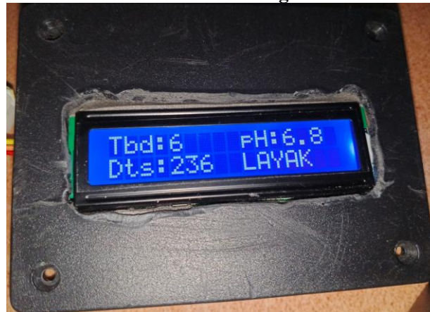
Figure 11. Test results with 3 water condition sensors
