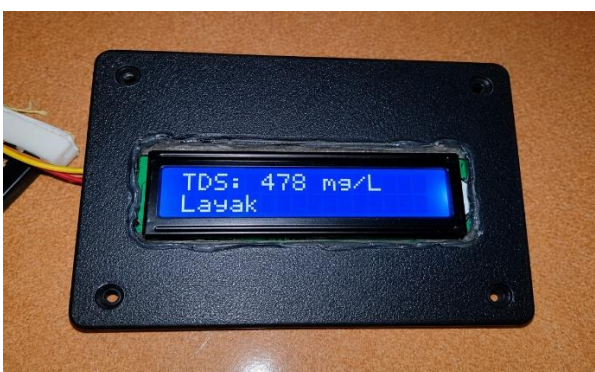
Figure 3. Test results for dissolved substances in water in a suitable condition
