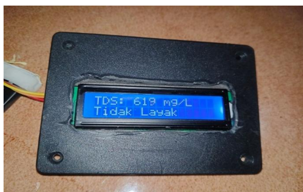
Figure 2. Results of testing dissolved substances in water in an unsuitable condition
