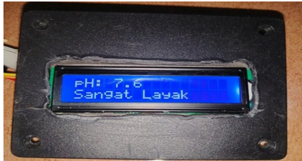
Figure 7. Test results if the water is not acidic and basic
